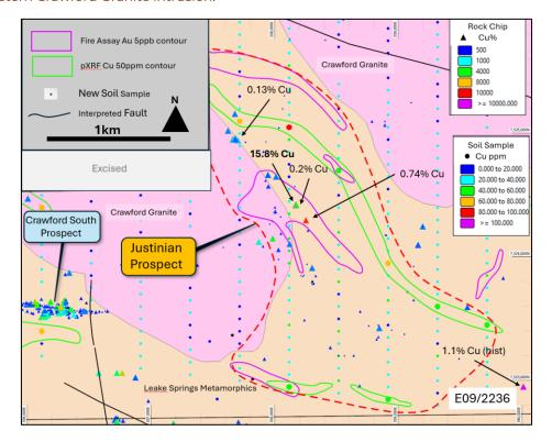
**Figure 4** Copper-in-soil results with new and previous rock chips from the Justinian Prospect. Both the Copper and gold anomalies appear to be following the trend of splays of the major Ti-Tree Shear as they wrap around the western Crawford Granite intrusion.
