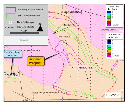
**Figure 3** Gold-in-soil results with new and previous rock chips from the 3.2km x 1.1km Justinian Prospect. Both the Copper and gold anomalies appear to be following the trend of splays of the major Ti-Tree Shear as they wrap around the western Crawford Granite intrusion.
