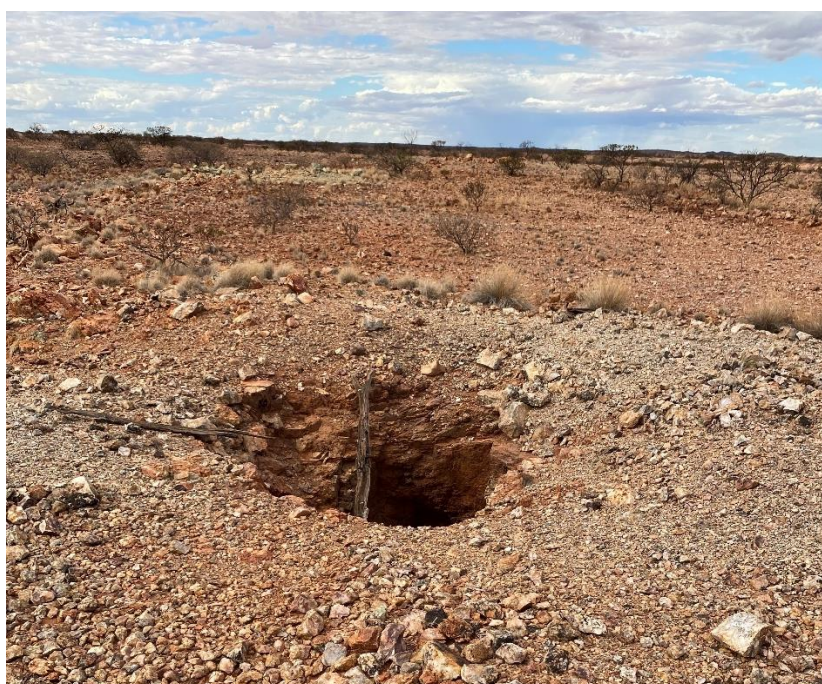
Figure 2 Shallow shaft at Tiberius with shallow workings and outcropping mineralised veins trending northeast.
