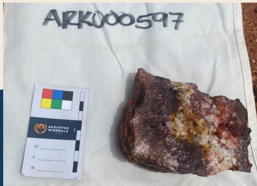
Dodd's quartz vein boulder sample which assayed 15g/t Au . ASX AUG Announcement 2 April 2025 "High Grade Mineralisation Continues at Music Well.
