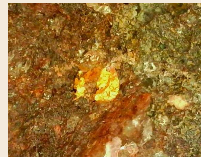
Visible gold in Dodd's quartz vein boulder sample (ARK000678) which assayed 122.8g/t Au. Width of gold grain is ~1mm. ASX:AUG Announcement 18 July 2025 "High Grade Vein with Visible Gold Discovered at Music Well".
