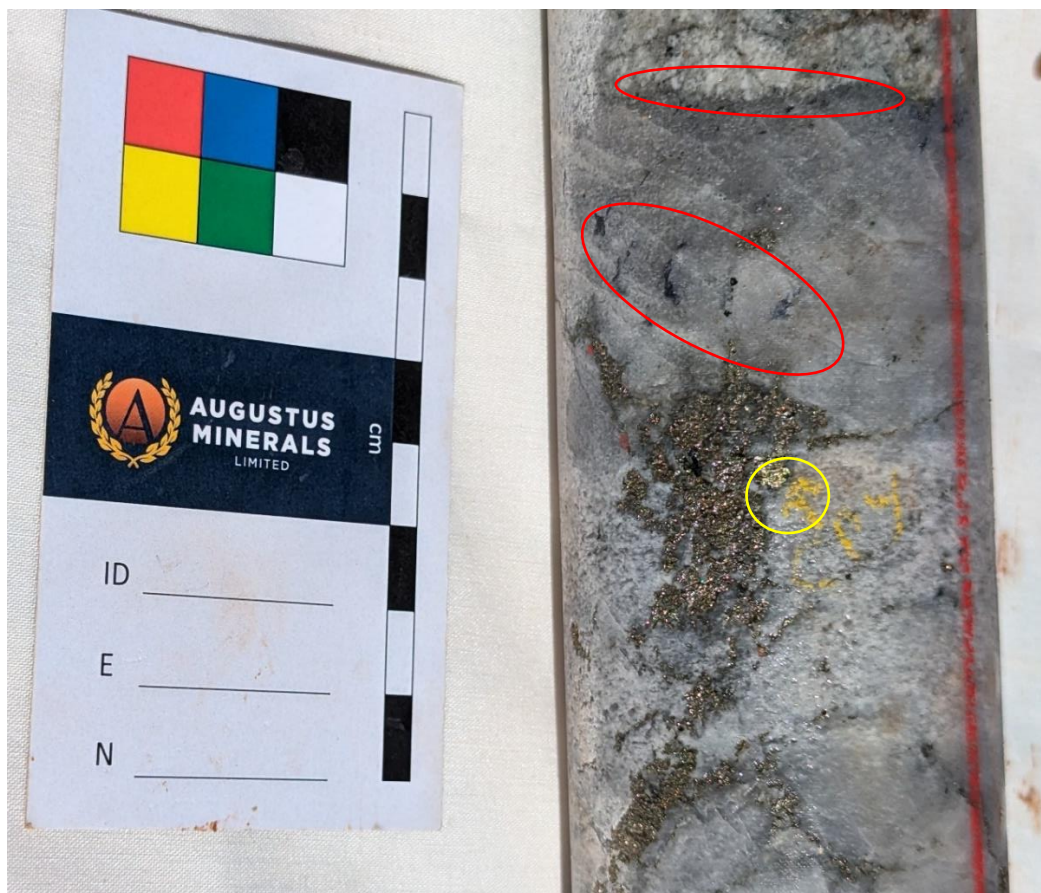
Figure 5 Grey molybdenite grains (red circle) and chalcopyrite bleb (yellow circle) within quartz vein with common brassy pyrite at 221.26m within interval averaging 5% pyrite, 1% molybdenite and 0.1% chalcopyrite from 221.00 to 221.6m. Yellow mark on core next to chalcopyrite in chinagraph pencil.
