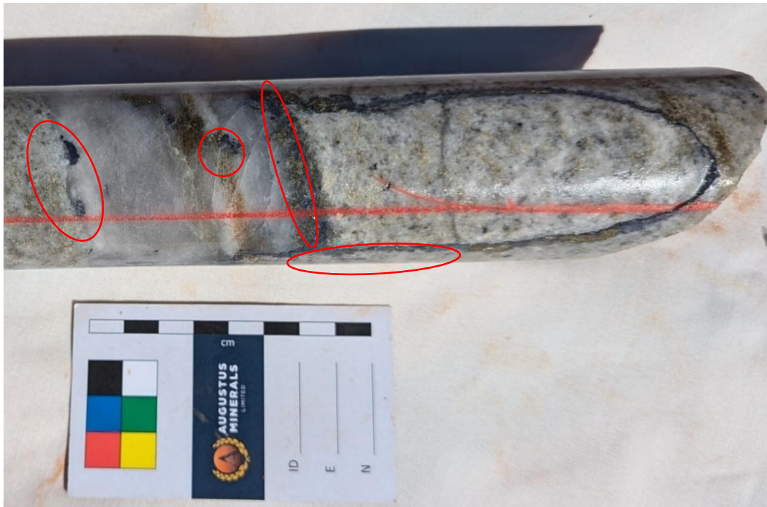
Figure 4 Grey molybdenite and brassy yellow pyrite in quartz vein and late chloritic shear/fracture at 261.6m within interval averaging 2% molybdenite from 261.54 to 261.82m.
