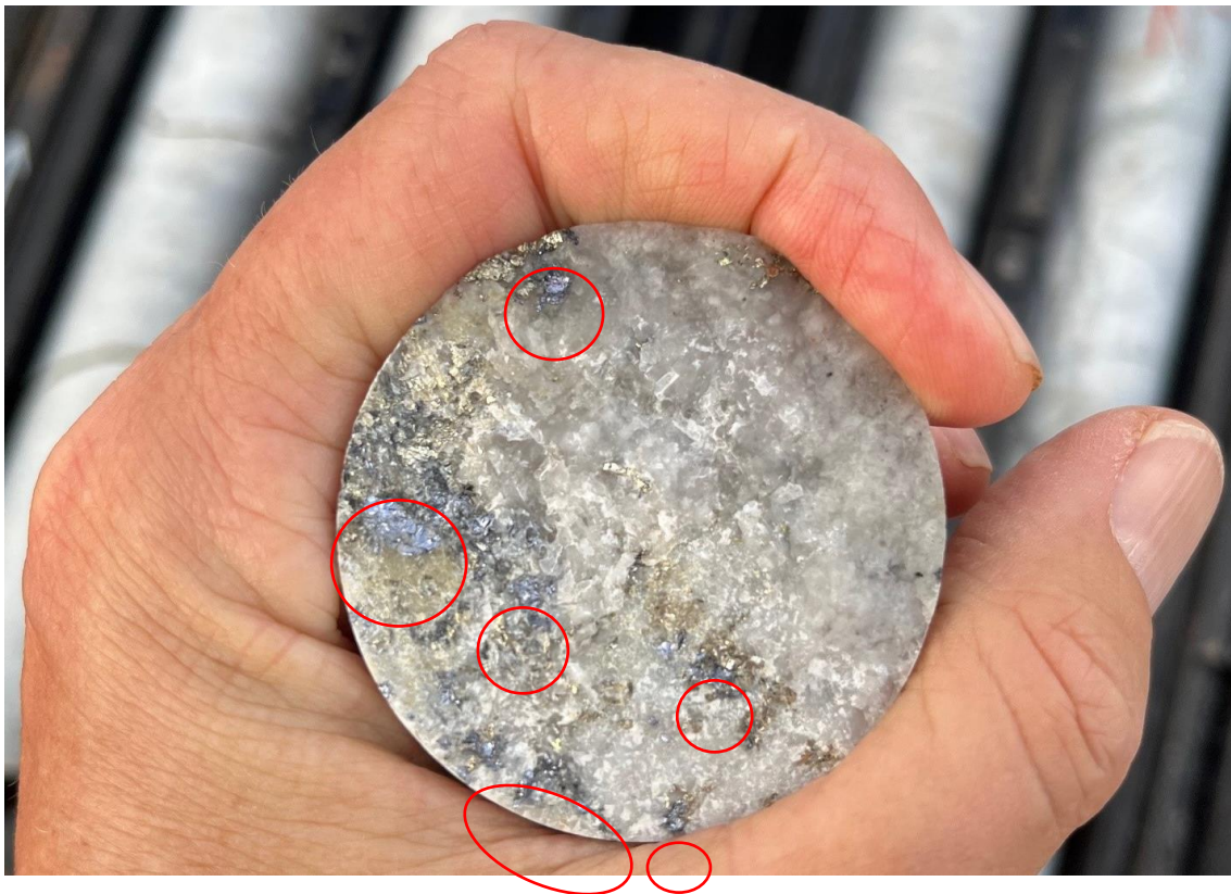
Figure 3 Blebby to disseminated pyrite (brassy yellow) and molybdenite (silver) (outlined in red) within a fracture on a quartz vein within MSD010 at 255.6m. This is within a zone from 255.41m to 255.72m averaging 3% pyrite and 1% molybdenite and 1% pyrite.
