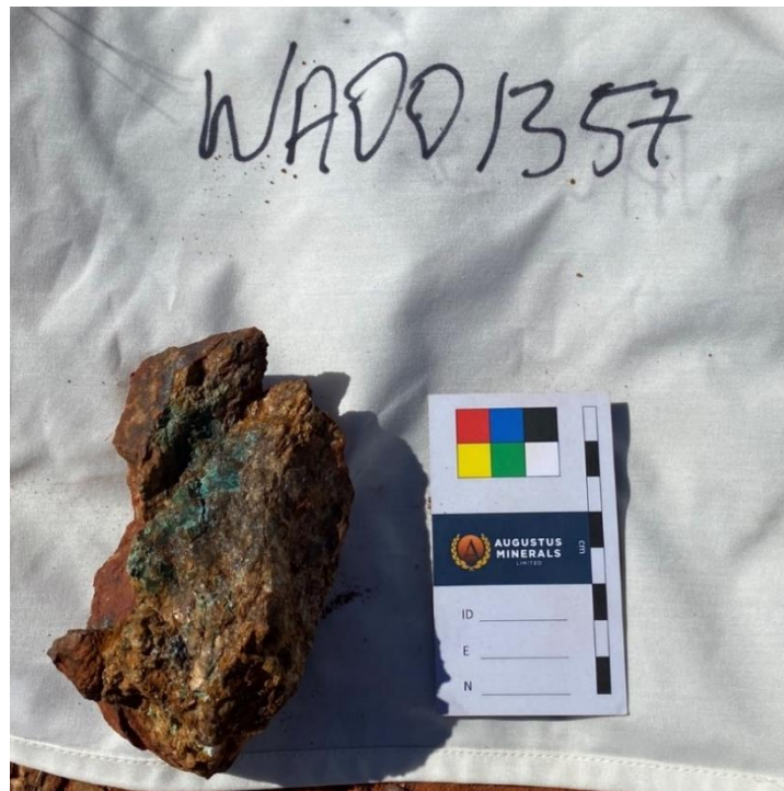
Figure 4 Photo of sample Wa001357 from a gossanous quartz vein with malachite which assayed 3.1% Cu .
