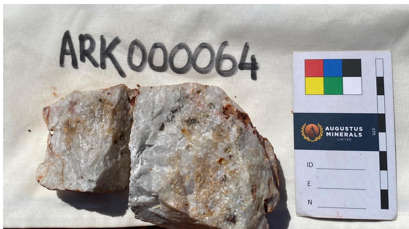
Figure 6 Photo of vein quartz from Augustus sample ARK000064 which assayed 50.1g/t Au at Clifton East. Note the brassy grey coloured fresh pyrite within the sample.
