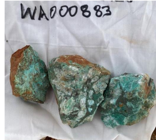
Copper rich brecciated quartz vein assayed 17.8% Cu, 65g/t Ag and 0.14g/t Au (Tiberius)
